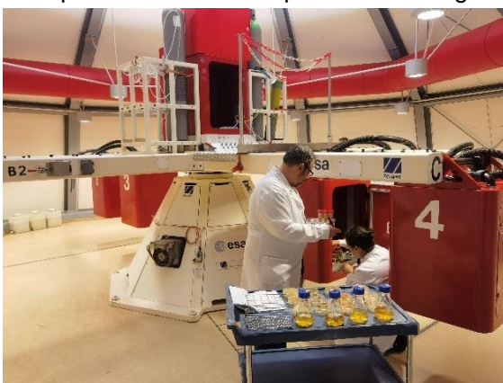
Marta and André were collecting samples from the Large Diameter Centrifuge (LDC) at ESTEC.
