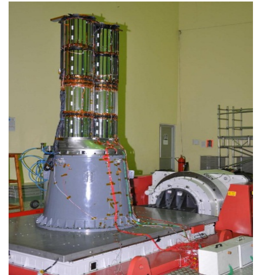
UVIT Payload Undergoing Vibration Test
