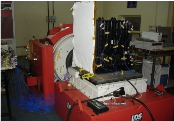
CZTI Payload undergoing Vibration Test
