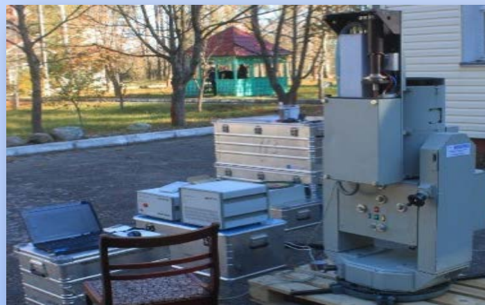
Equipment for determining the optical parameters of the atmosphere at test ranges
