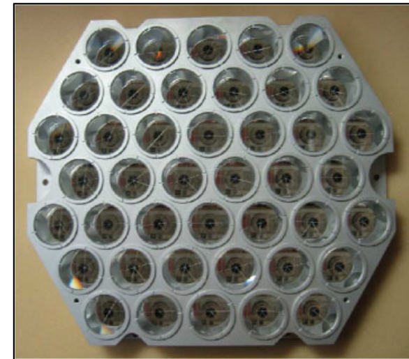
Beidou laser retroreflector array (31.6 x 28 cm, planar, hexagonal array; 2.5 kg) (Chinese Academy of Sciences)
