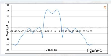
GNSS Transmitting antenna gain pattern
