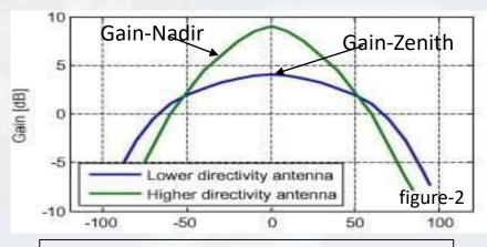
GNSS Receiver antenna gain pattern
