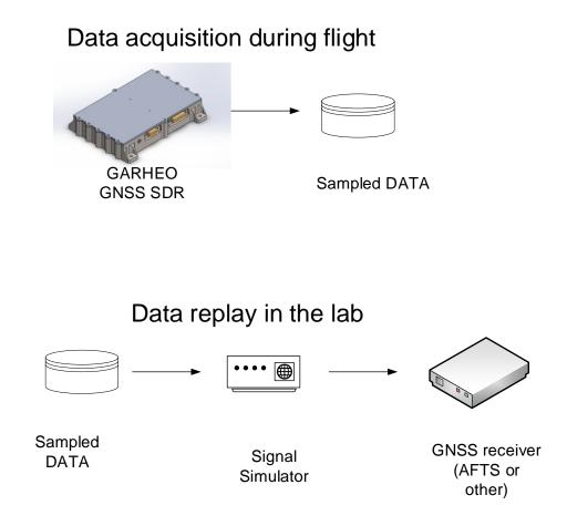
A space designed SDR electronics has been developed with specific requirements for the high accelarations and vibrations of the sounding rocket
