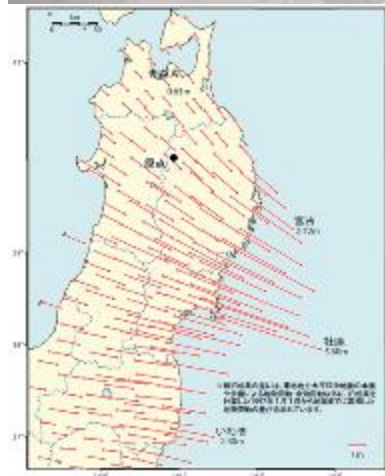
Local survey coordinate has a gap with GNSS coordinate (ITRF).
