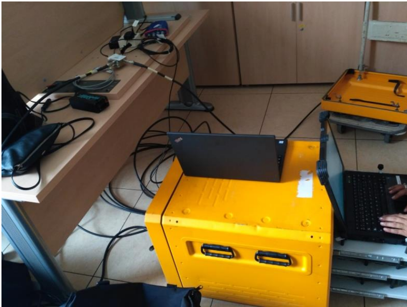
ENAIRE's GNSS/GBAS portable monitoring station.
