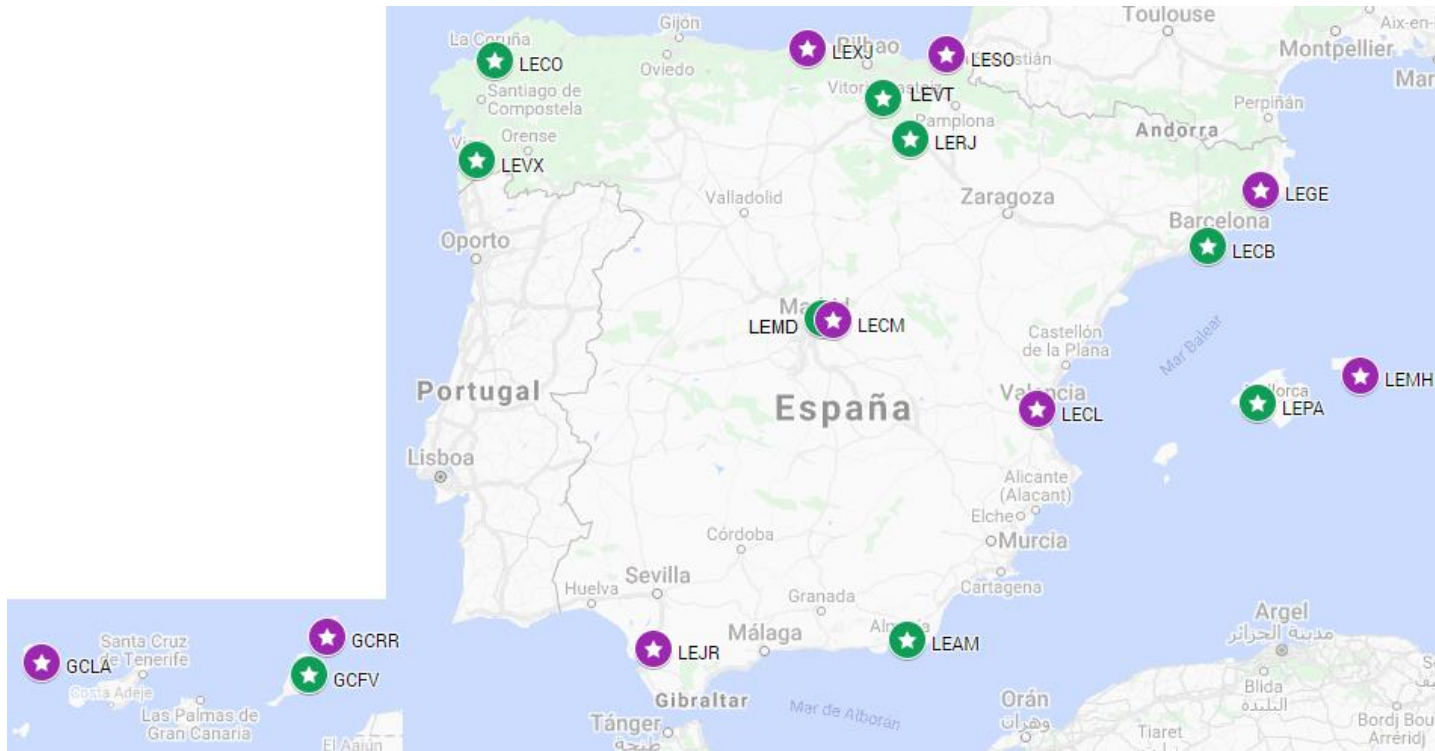
Green color: GPS/Galileo L1/E1/L5/E5a monitoring stations. Purple color: GPS L1 monitoring stations.
