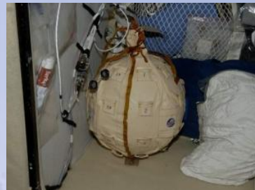
Matroshka: study of radiation environment with different phantoms in- and outside ISS
