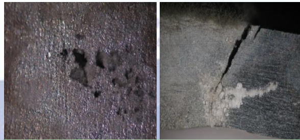
Corrosion of aluminum alloy under combined action of ultrasound and water condensate (x 200)
