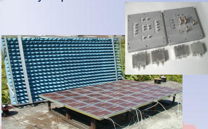
8 – channel microwave radiometer ( \lambda = 21 \text{ cm} )
