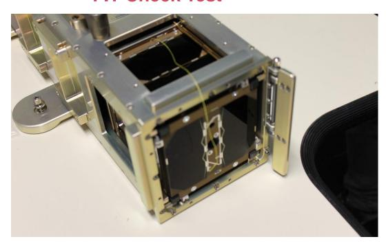
Inside the J-SSOD orbital deployer
