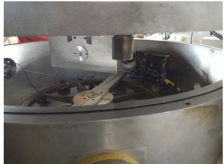
Heavy-ion damage tests of FPGA-based SpaceWire component in the Pelletron Accelerator of USP
