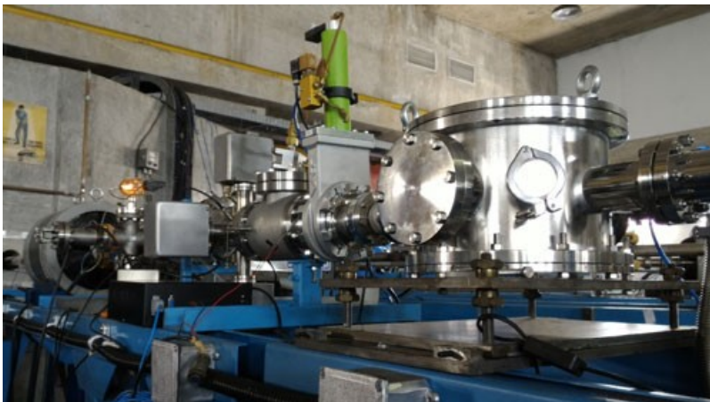
Heavy-ion damage tests of FPGA-based SpaceWire component in the Pelletron Accelerator of USP
