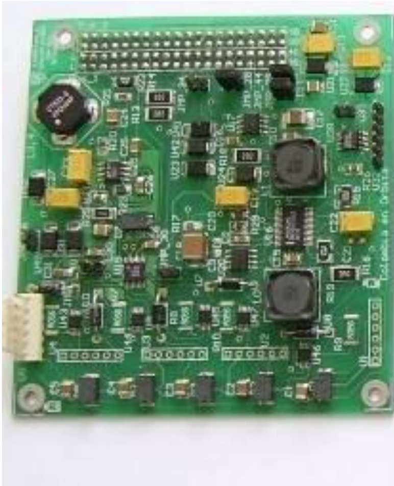
Electrical Power Supply
