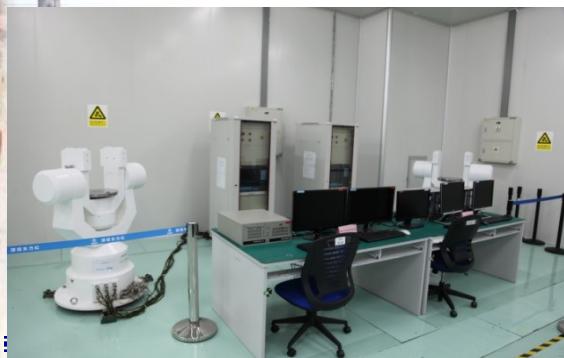
3 meters semi-anechoic chamber
