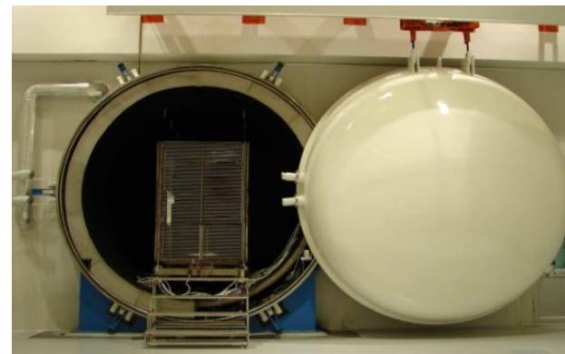
\Phi 3.6\text{m} \times 5\text{m} Thermal Vacuum Environmental Test Facility
