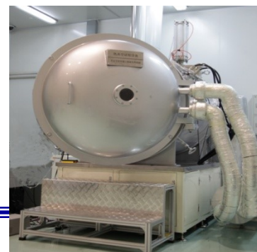
\Phi 3.6\text{m} \times 5\text{m} Thermal Vacuum Environmental Test Facility
