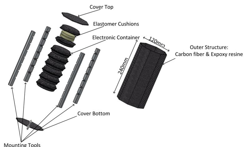
Figure 3: Exploded view of  $\eta$ Sat-IE
