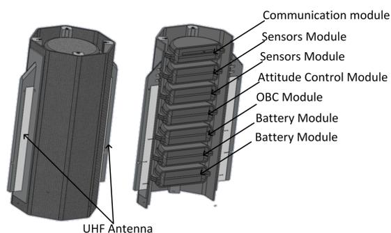
Figure 1: Structural configuration for orbital mission
