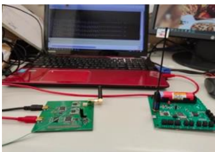
(Top) 400/433MHz LoRa receiver. Simplified version of the LoRa receiver on board the KITSUNE satellite ©Fatima Duran (Bottom) Checking communication between the LoRa receiver and Ground Sensor Terminal (GST) ©Pooja Lepcha
