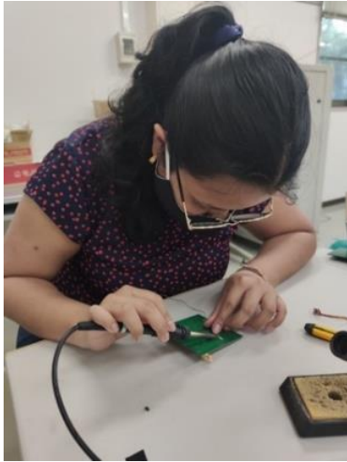
Soldering some components of the LoRa receiver ©Pooja Lepcha
