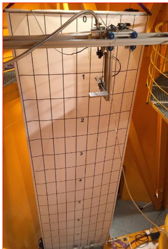
Figure 5-8 The scale net mounted in the background
