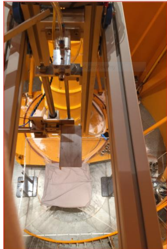
Figure 5-5 Mounting the ERS on the handrail of deceleration chamber – on the right picture the secure mesh and the secure “pillow” are visible
