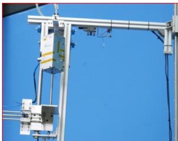
Figure 5-2 ERS – the plate in a down position, DM is hanging now on a wire
