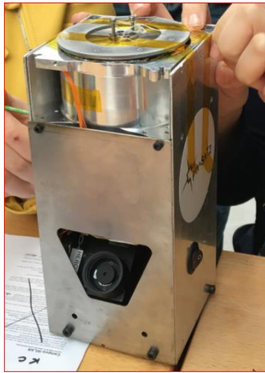
Figure 4-1 The dummy model of the PW-Sat2 satellite manufactured on purposes of DropTES campaign
