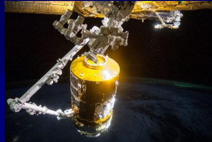
Docking of “Kounotori” to ISS by robot arm
