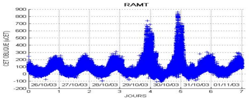
**Oblical Total Electronic Content at RAMT station (USA), during a ionospheric perturbation**
