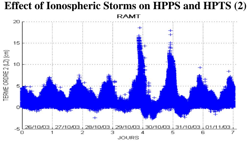
Ionospheric 2<sup>nd</sup> order pseudorange term at f<sub>NA</sub>1 GPS frequency calculated for the RAMT station
