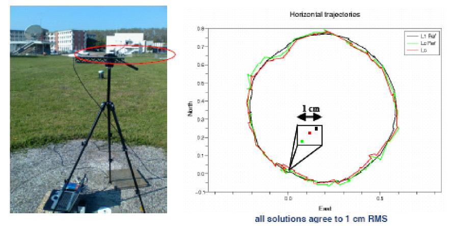
Accuracy close to 1 cm provided by PPP-WIZARD using GPS signals at  $f_{NA}$ 1 and  $f_A$ 3 frequencies. PPP-WIZARD : PPP With Integer Zero-difference Ambiguity Resolution Demonstration
