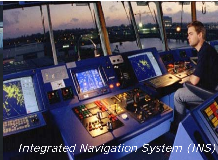
Integrated Bridge System (IBS)
