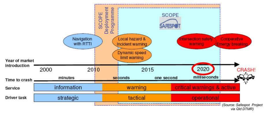
Use of Positioning in Vehicles is going from Passive to Active... from simple navigation to information about traffic to warnings about hazards to actively avoiding hazards.
