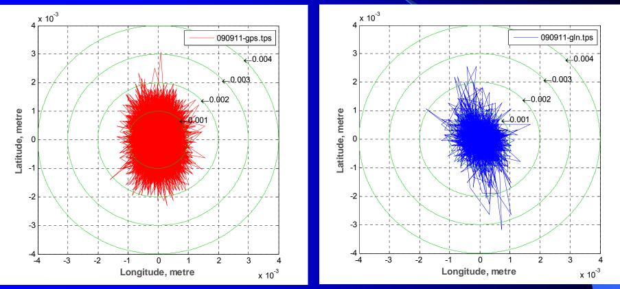
Accuracy of GLONASS RTK positioning is the same as GPS RTK accuracy provided enough number of GLONASS satellites are available for positioning
