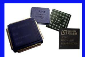
Components of BeiDou/GPS dual-mode vehicle terminal
