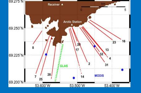
Ground tracks of the reflected GPS signals (with PRN number) obtained during raw acquisition for the whole campaign (red lines). Positions of GLAS and MODIS data samples are marked with green and blue respectively. White triangles mark the location of the receiver and the Arctic station.
