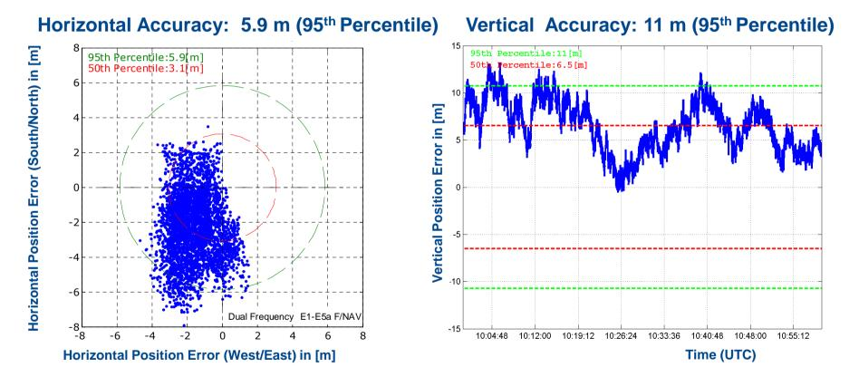
Position Fix established with Test User Receivers in real-time and with TGVF Reference Receivers off-line.
