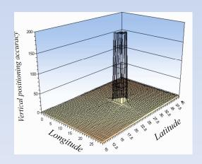
Vertical positioning accuracy degradation and sizes of degradation zones
