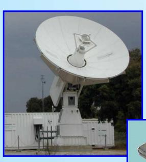
ViaSat (5,4 m fixed X-band tracking system): • diameter 5,4 м; •gain factor G/T 31,5 dB/K (typical)
