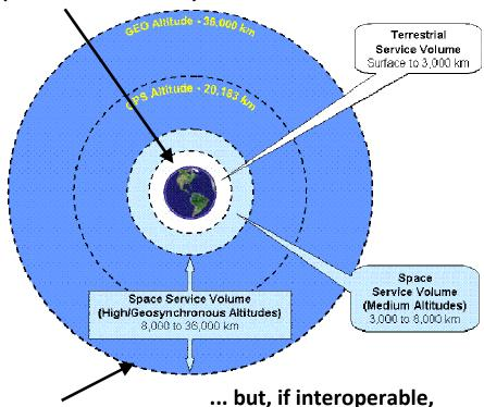
Only 1-2 GPS satellites in lineof-sight at Geosynchronous orbit altitude then GPS + Galileo +
