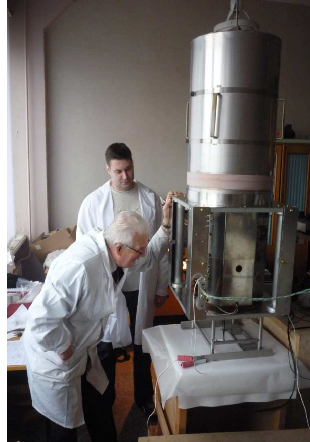
Assembling of the fountain mainframe & magnetic shield
