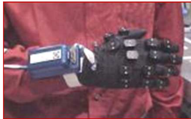
Posture Acquisition Glove (PAG) and Wrist Electronics Box (WEB)
