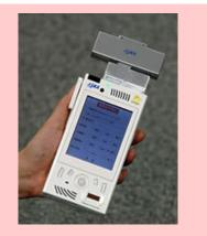
Handheld Terminal (300 g) 50 – 400 bps (TX) 1.6 kbps – 12.8 kbps (RX)
