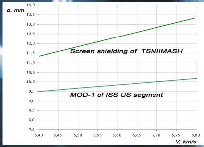
Experimental data comparison on ballistic limit curves of ISS US segment shielding MOD-1 and TSNIIMASH shielding
