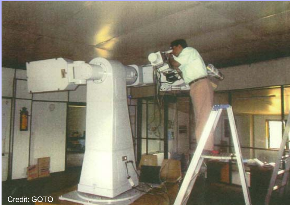
Sri Lanka astronomer adjusting CCD spectrograph for the reflector.
