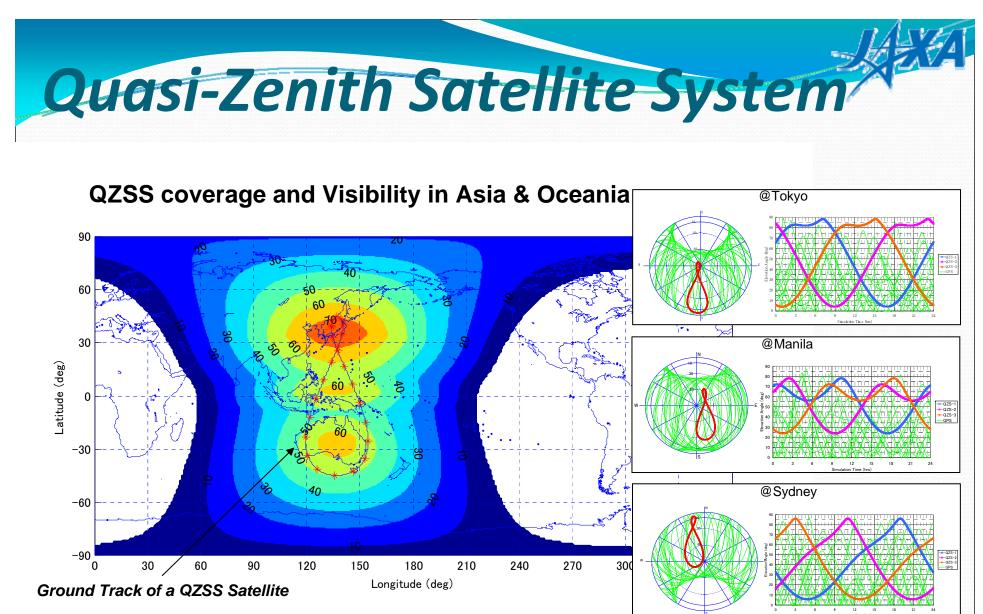
At least one QZSS satellite can be observed more than specified elevation angle any time. For instance, users in orange colored area can receive at least one QZSS satellite with 70 degrees or more.
