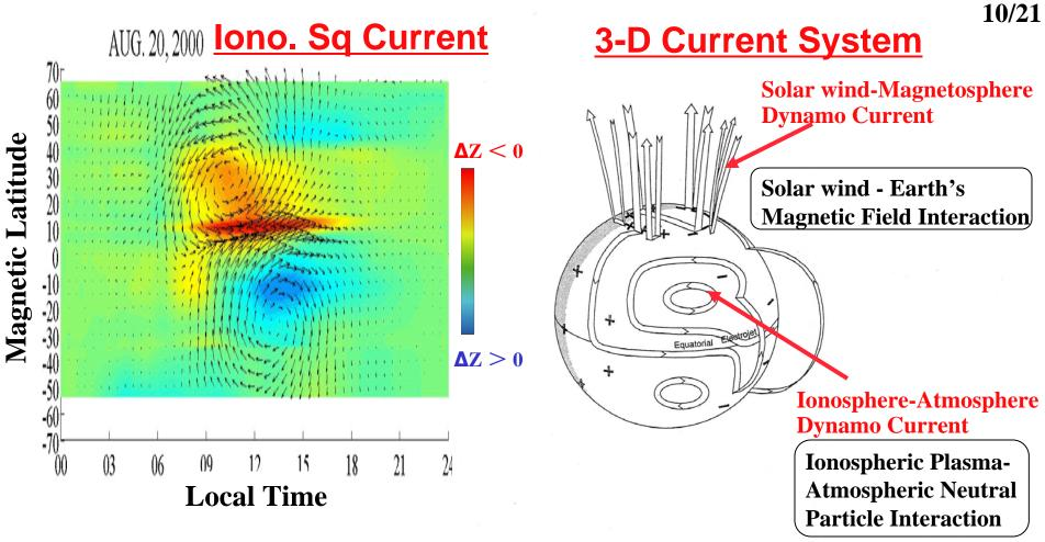
(left) Global equivalent ionospheric current pattern obtained by the ordinary MAGDAS/CPMN data. (right) Three-dimensional current system in geo-space.
