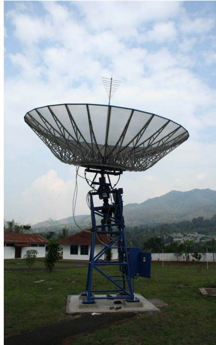
SOLAR RADIO SPECTROGRAPH - SN 4000 RADIO SPECTRUM : 18 MHz – 1.8 GHz OPERATING NOW: 56 MHz – 1.8 GHz
