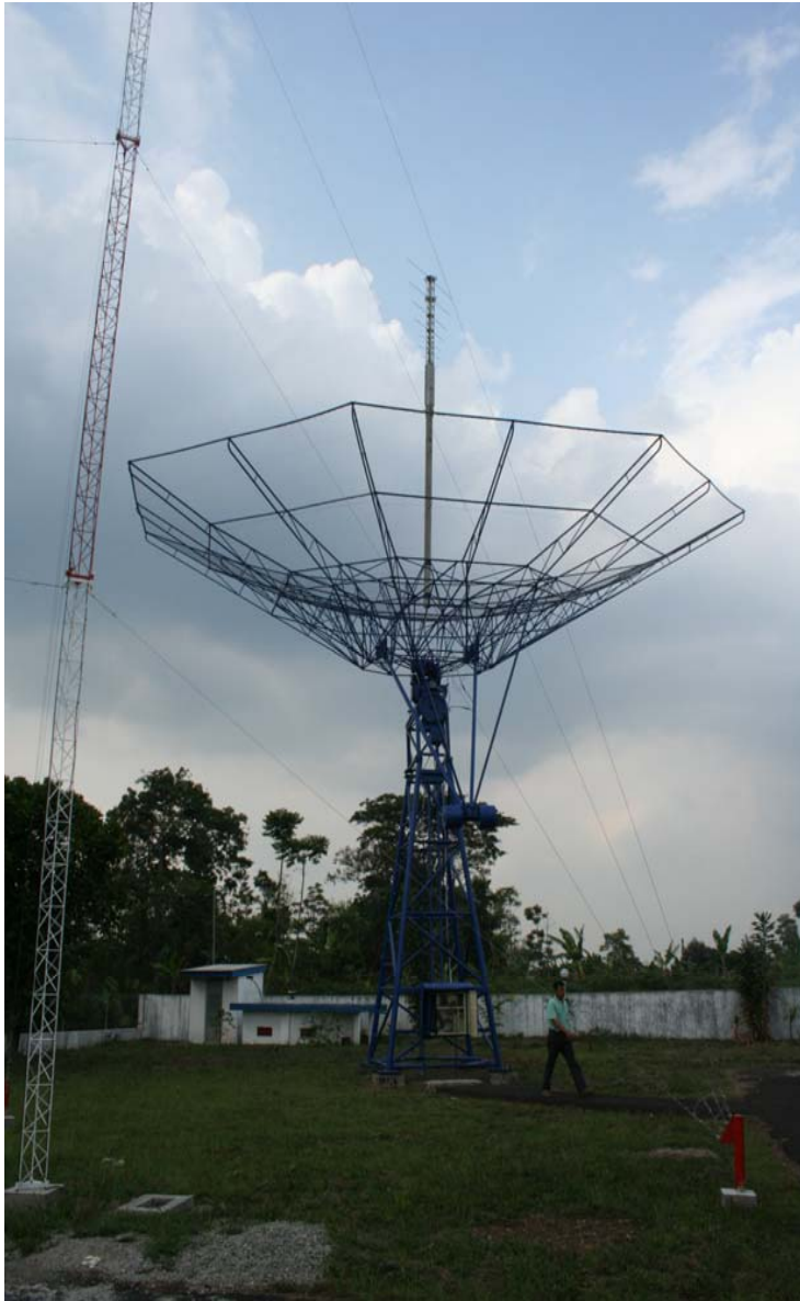
SOLAR RADIO SPECTROGRAPH - SN 4000 RADIO SPECTRUM : 18 MHz – 1.8 GHz OPERATING NOW: 56 MHz – 1.8 GHz
