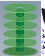
A modular deployment system for double and triple CubeSats
