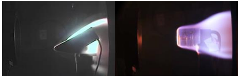
Fig. 6 Evaluation Tests by Arc Heating Wind Tunnel
