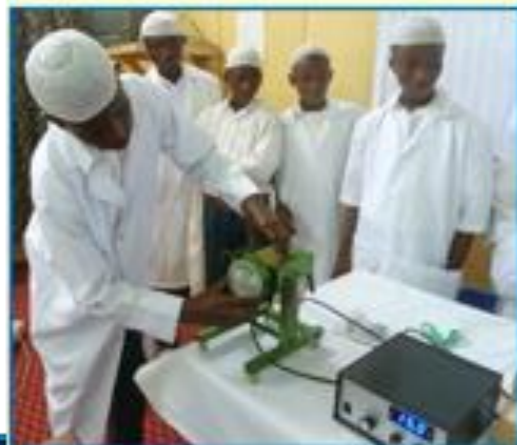
Mounting the sample on the Clinostat
