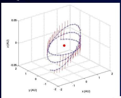
Asteroid 2011MD (200 ton class) Thrust = 15N ON/OFF profile → 985 days to L2
