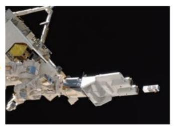
The robotic arm of "Kibo" holds the MPEP to transfer it to the release point. The satellites are deployed by a command signal sent from ground.
