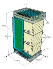
LIDAL (Light Ion Detector for ALTEA) is a particle detector based on the ASI payload ALTEA. It has improved features such as detectors based on scintillators and fast electronics. Its objective is to study and characterize cosmic radiation on board the ISS. LIDAL will allow:
