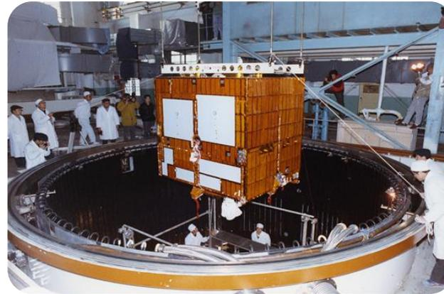
Thermal vacuum chamber 7m(Diameter)\*12m(Height)
