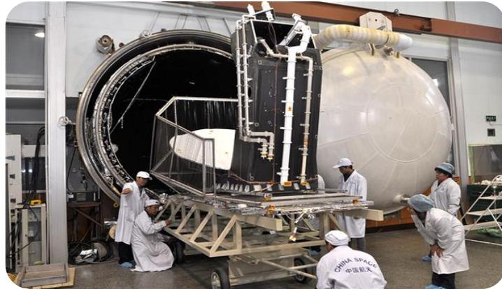
Thermal vacuum chamber 3.6m(Diameter)\*5.5m(Length)
