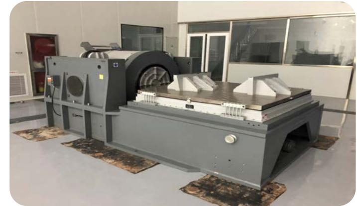
200kN Shaker for Vibration Test
