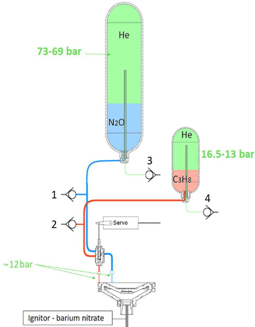
**Scheme of the propellant supply system for a rocket engine:**
