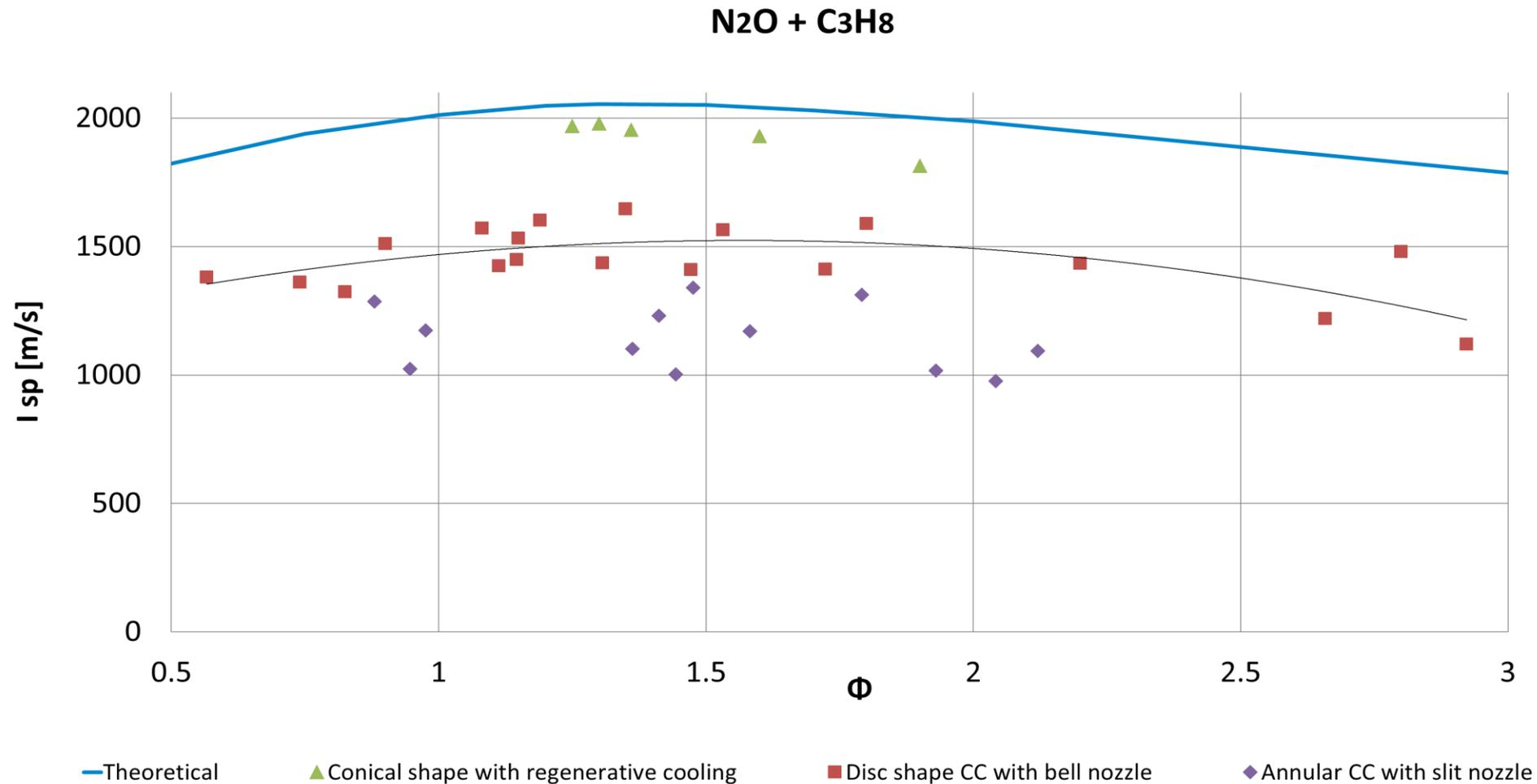
**Specific impulse in different shape detonation chambers for different mixture composition. Red points – disk-shaped combustion chamber, purple points – annular combustion chamber, green points – experiments with cone shape chamber with regenerative cooling system. Blue line shows theoretical specific impulse calculated by NASA CEA Code**
