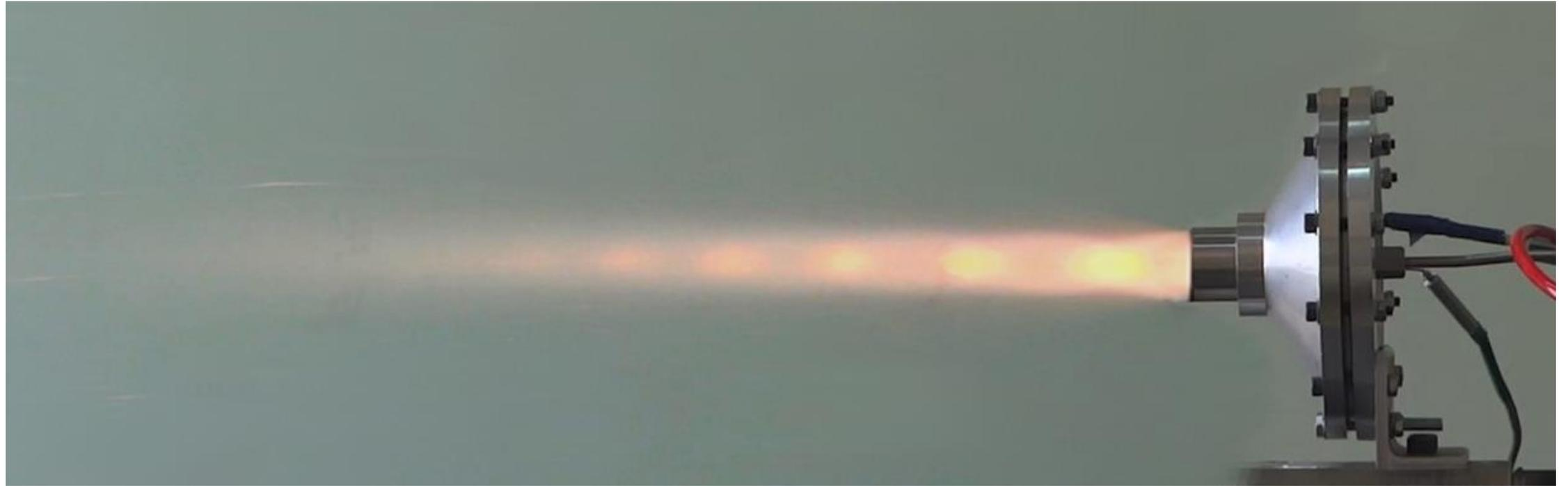
**Detonative rocket engine, supplied by liquid propane and nitrous oxide ( $C_3H_8-N_2O$ ) tested at the Łuksiewicz-Institute of Aviation in Warsaw**
