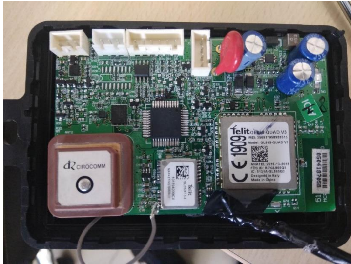
NavIC based VTS for AIS-140 testing (NavIC module by Telit) Brandname: Autocop
