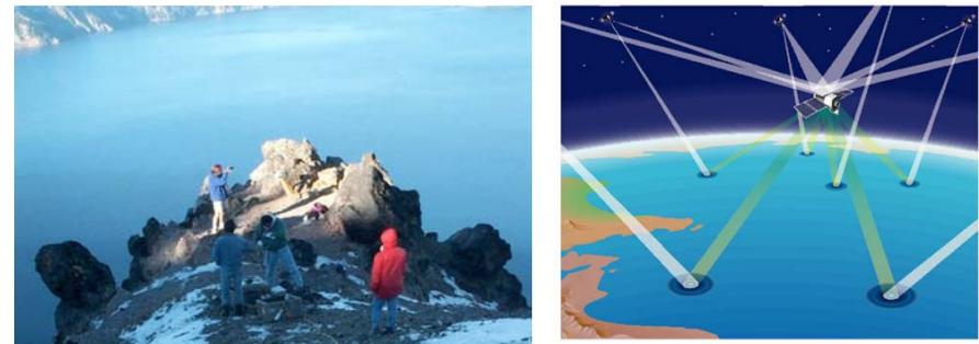
**2 cm precision altimetry in 1-sec using phase from fixed receiver (Crater Lake, OR)**
