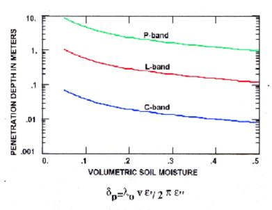
Penetration depths calculated as a function of volumetr moisture for C-, L-, and P-band assuming a sandy loam soil consist 51.5% sand, 35% silt and 13.5% clay (Ulaby et al., 1986).
