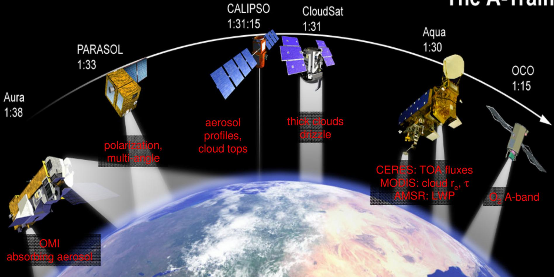
The Afternoon Constellation consists of 7 U.S. and international Earth Science satellites that fly within approximately 30 minutes of each other to enable coordinated science. The joint measurements provide an unprecedented sensor system for Earth observations.
