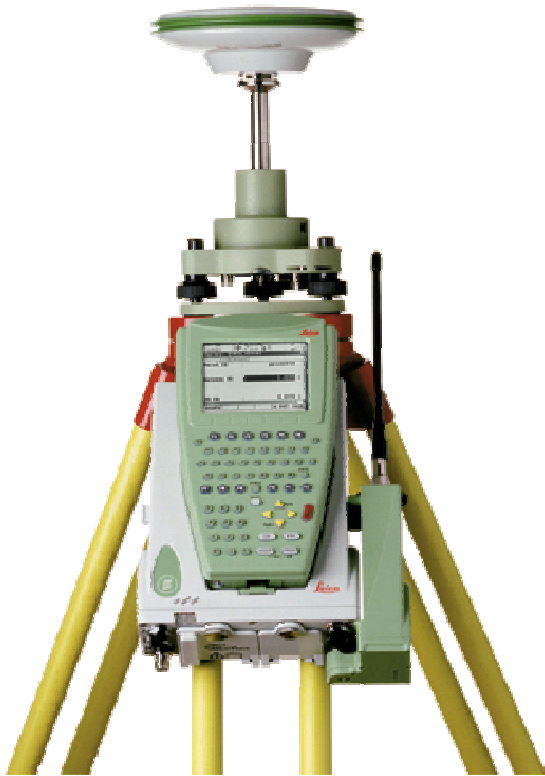
Temporary GNSS Base Station
