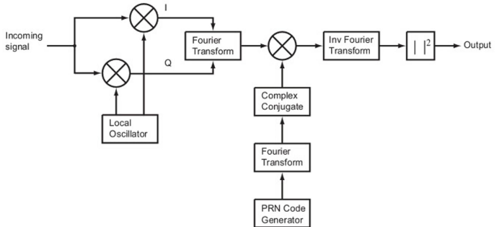
Schematic representation of FFT based acquisition
