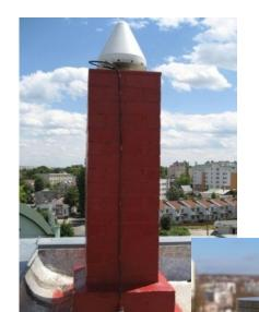
In 2007 the Agency, in collaboration with Bundesamt für Kartographie und Geodäsie (BKG), EUREF and EuroGeographics, has installed and jointly operate the first GNSS permanent station IGEO in Chisinau. This reference station is integrated into the EUREF Permanent Network (EPN) and the International GNSS Service array (IGN).
